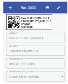
box label and registration date, as stored on the FreezFiler Server. The labels can be either sticked to the side of the box, as mandated in many laboratories, or on a paper labbook. The labels also contains a QR code, to allow quick retrieval of the box metadata using the FreezFiler App.
